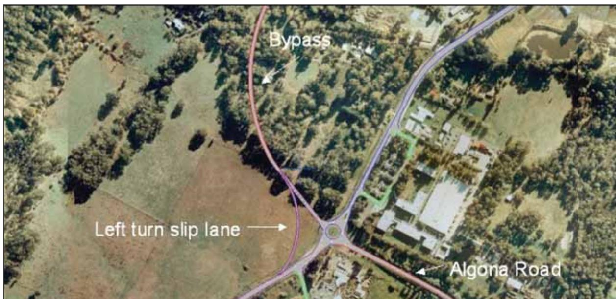
**Figure 9** Bypass Option BP10 with Left Turn Slip lane at Algona Road
